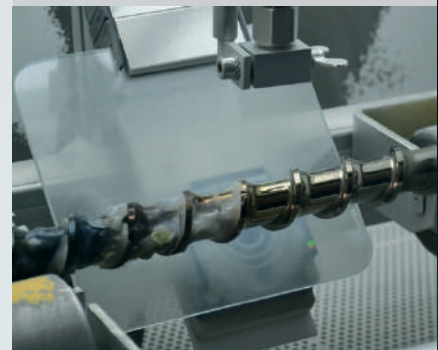
Screw-segment before and after cleaning process
